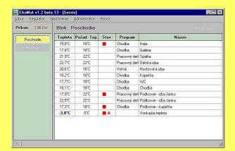
This application EKOMAT allows effective use with temperature control system DUEL. Through the application can monitor the current room temperature, as heating elements, desired parameters etc., directly on your PC screen and gain visibility across the heated object.
