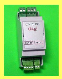
DX4101.DIN controller is designed for solar thermal systems with one circuit, which provides automatic control system operation.
